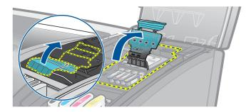
4 Lift up the handle of the printhead and use it to pull the printhead straight up and out of its slot.
